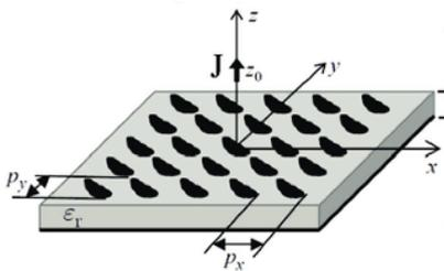
Fig. 1 Example of a periodic metasurface from [1].
